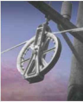
Twisted Pair conductors stringing sheave
